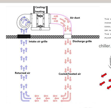
THE WORKING PRINCIPLE OF FAN COIL UNIT IS TO SEND INDOOR AIR OR OUTDOOR MIXED AIR INTO THE ROOM AFTER COOLING OR HEATING THROUGH THE COIL, SO AS TO REDUCE OR INCREASE THE INDOOR TEMPERATURE.
